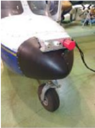
Figure 6. – ATLAS multisensory box integrated on the fore part of the PIXAIR airplane structure
